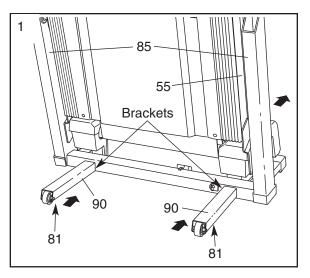
With the help of a second person, carefully tip the Frame (55) and the Uprights (85) down to the position shown.
